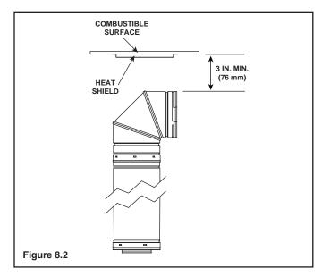
Fasten the shield in place using the four pilot holes provided in the part.
